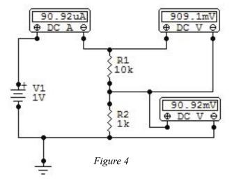
divided by a factor of 1 plus the ratio of the resistors. You can visualize this easily with a simple 1:1 divider; two equal-value resistors. By inspection you already know that the input voltage will be divided by two. The division ratio is 2, which is 1 plus the ratio of the resistor values. Revisiting the 10:1 voltage divider:
