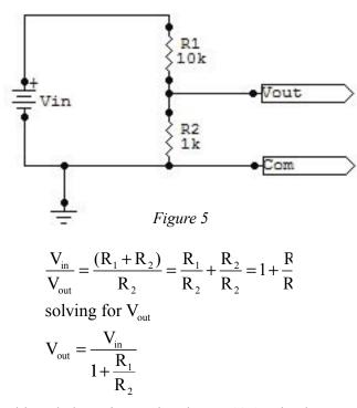
although the resistor values have a 10:1 ratio, the actual voltage division was 11:1. To obtain a 10:1 division ratio, the resistors must have a 9:1 ratio.
