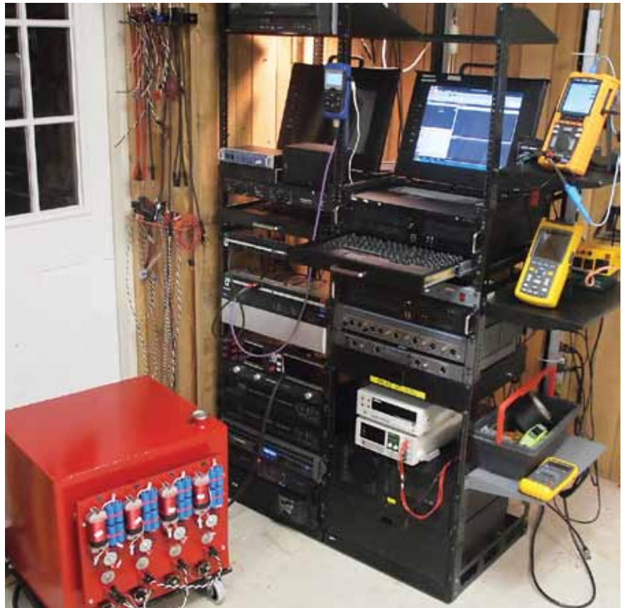
Figure 1: Inside the testing - four 1,800-watt water heater elements (purely resistive) mounted into a 25-gallon steel tank.
