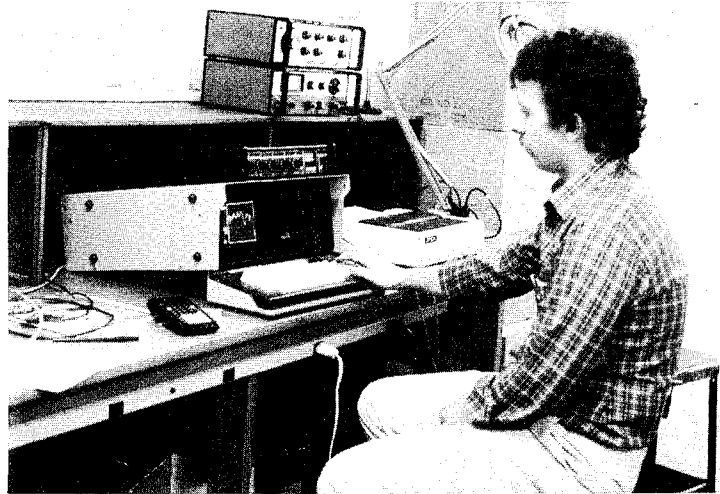
J. W. Davis engineer, Gary Boyd, using their TEF® analyzer for loudspeaker measurements.
